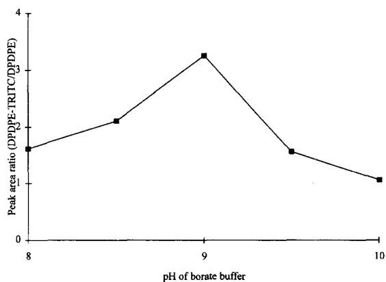
Fig. 10. Buffer pH optimization for DPDPE derivatization with TRITC. Conditions were as described in Section 2.2.3.
